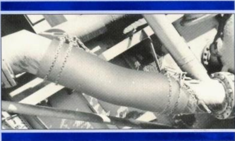
Type SDS soft-wall 12 \frac{3}{4} -in. stern discharge hose.
